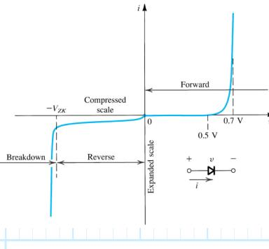
Note that the breakdown region occurs when the junction diode voltage (from anode to cathode) is **approximately** less than or equal to a voltage value  $-V_{ZK}$ . The value  $V_{ZK}$  is known as the **zener breakdown voltage**, and is a fundamental performance parameter of any **junction** diode.
